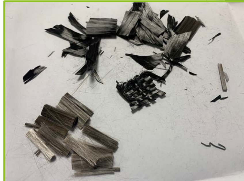
After: Pristine carbon and glass fibres ready for repurposing
